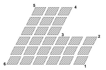
It is not necessary to take measures at each panel corner, for example, in the case of staggered panels. Shade measurements should be made at the major corners of the array as shown below.
